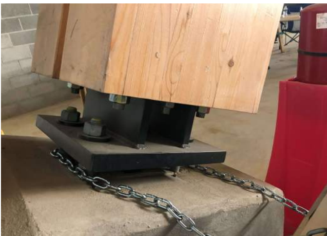
Heavy timber steel connection system.
