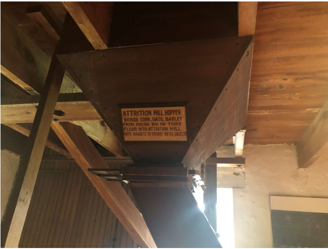
Hopper Used To Transfer Grains To Lower Level Floors
