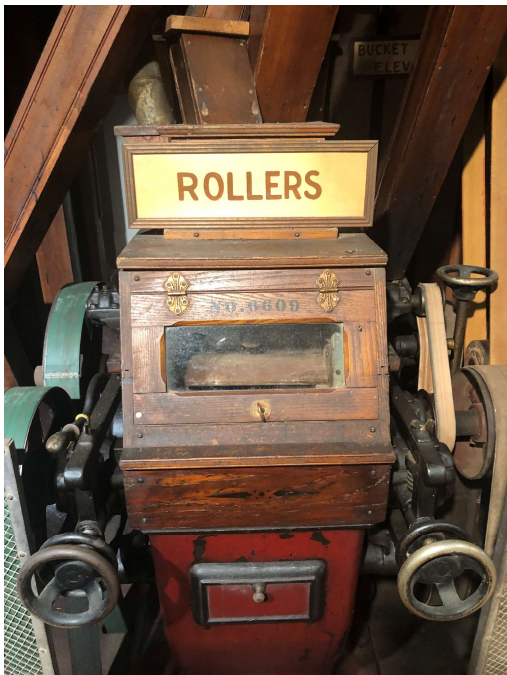
Rollers Used In The Process Conversion of Wheat to Flour.
